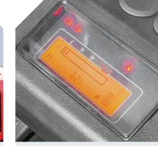
Newly-developed LCD instrument has more comprehensive functions and more stable performance and entirely displays the full truck state, fault code and other important information, which can make the operator more intuitively and conveniently have a better knowledge of truck state and make the maintenance conveniently.
