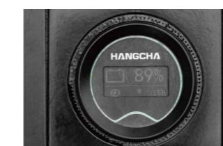
The integrated power display, timing, and fault self-diagnosis table are convenient for maintenance.
