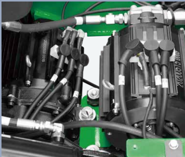
Both the traction and oil pump adopt permanent magnet synchronous motors for the Enpower controller
